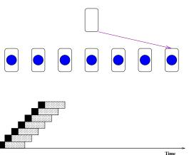
ssh pipeline shift: 5msExecution time:  $n \times 5ms + 95ms$ For 1000 nodes: 5, 1*s* Gain is about 100/5 = 20(constant factor)
